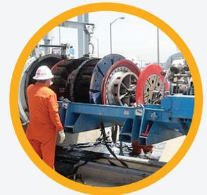
A "smart pig" being readied for an internal pipeline inspection
